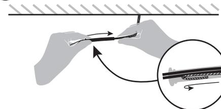
5 Fold the yellowgreen ceiling wire and insert all the ceiling wires through the rubber sleeve.
