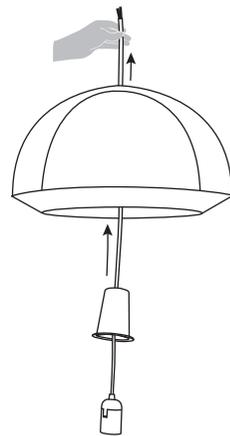
2 Thread the cord through the lampshade from underneath.
