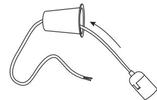
1 Thread the cord through the cone-shaped cup.
